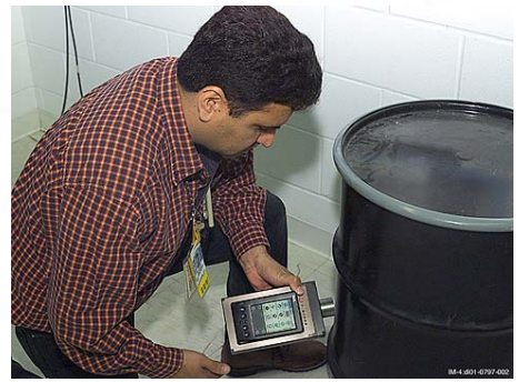
Handheld nuclear material detector locates and identifies isotopes
